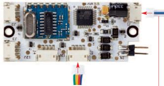
Green cable = to Lighting Output Yellow cable = to Lighting Output Red cable = to Lighting Output Blue cable = shared Common/Ground Wire White cable = to Lighting Output Blue cable = shared Common/Ground Wire White cable = to Lighting Output
